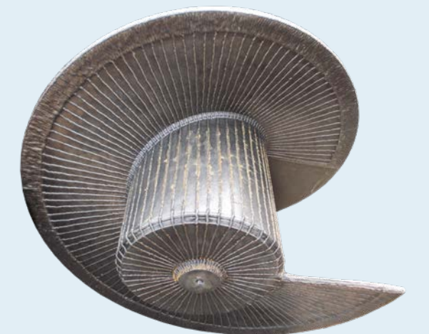
Screw conveyor shaft with wear protection for power stations
