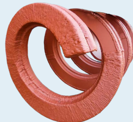
Screw conveyor shaft with wear protection for the glass industry
