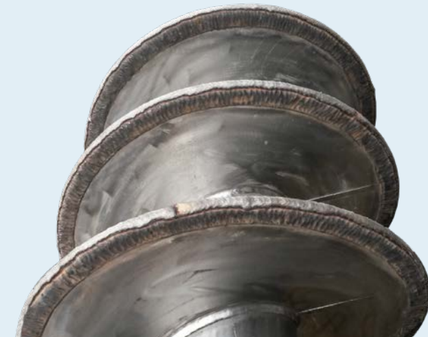
Screw conveyor shaft with wear protection for the sugar industry
