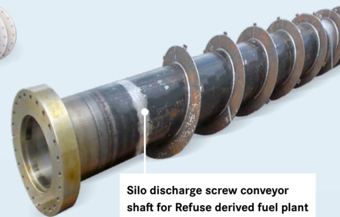
**Silo discharge screw conveyor shaft**
