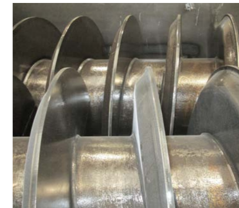
2. Double cooling screw conveyor
