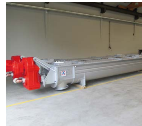
1. Trough cooling screw conveyor
