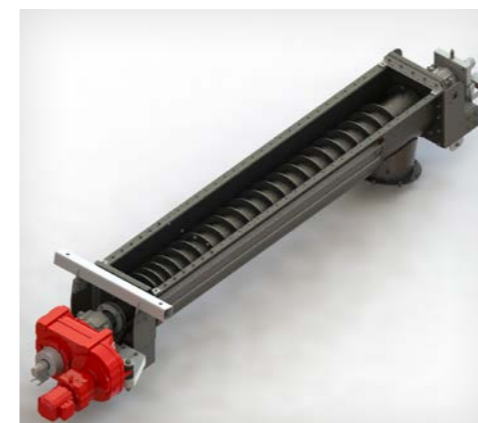
3. Trough cooling screw conveyor
