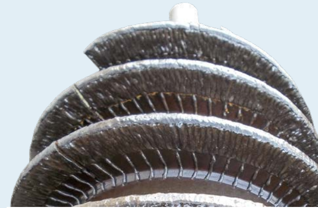
Screw conveyor shaft with wear protection for power stations
