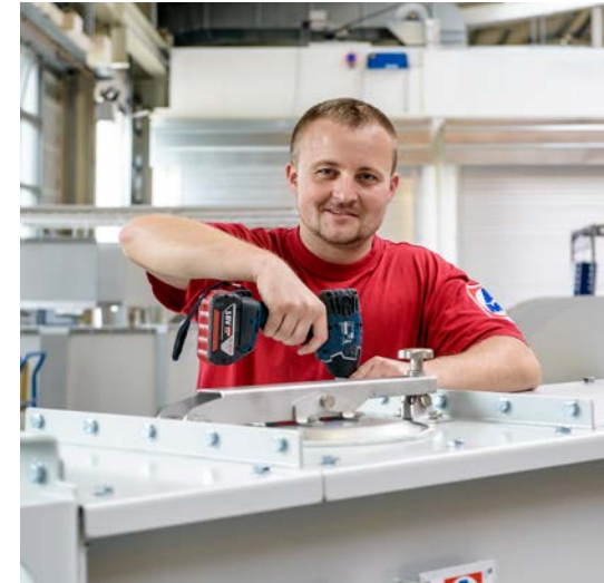
Final assembly of an AMF-Bruns trough screw conveyor
