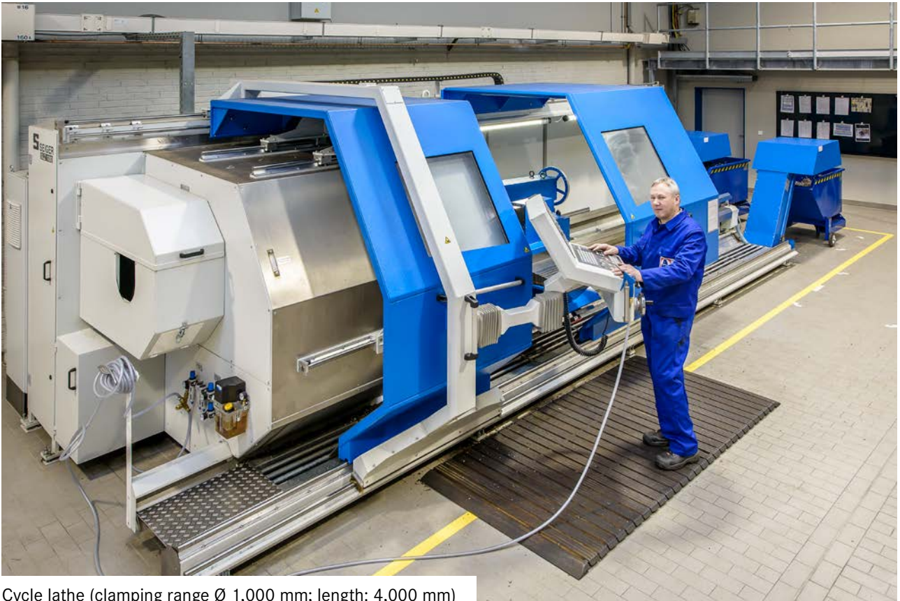
Cycle lathe (clamping range Ø 1,000 mm; length: 4,000 mm)
